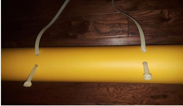
2. Attach the launch tube to the trailer at a 45 to 60 degree angle pointing at the boat, as seen below. Find a place to affix the tie wraps on the winch post opposite from the winch crank.
