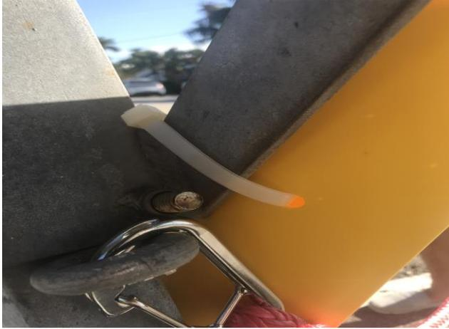
4. Attach the shock absorber end to the bow cleat of your boat.
