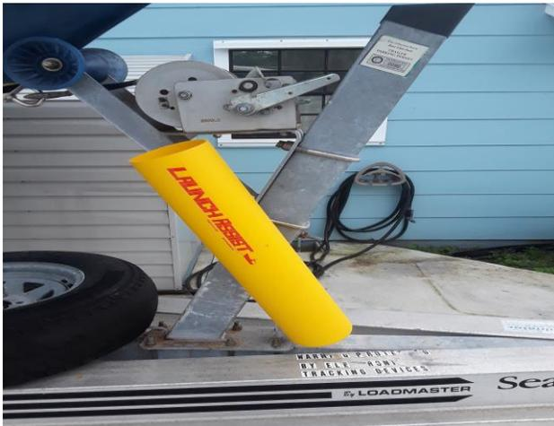
3. Attach the rope end stainless spring hook to a fixed loop on your trailer as seen below. If you do not have a secure place on your trailer, you can use a 1/2 inch or larger galvanized welded eye bolt. You should 1st measure the depth of your winch post or trailer frame to make sure it goes all the way through with a nut on the other side and a washer on both sides.
