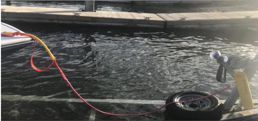
8. After launching your boat, you can use Launch Assist as a dock line with a built in shock absorber! Simply detach the rope end from the trailer and tie off on the cleat.
