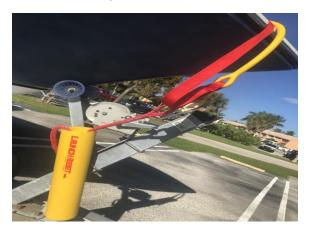
6. Before launching your boat, be sure to detach your winch strap and double check to make sure that the Launch Assist line is securely attached on both the boat and trailer.
