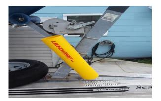
3. Attach the rope end stainless steel spring hook to a fixed loop on your trailer as seen below. If you do not have a secure place on your trailer, you can use a 1/2 inch or larger galvanized welded eye bolt. You should 1st measure the depth of your winch post or trailer frame to make sure it goes all the way through with a nut on the other side and a washer on both sides.
